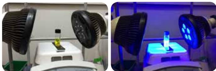
**Figure 4. Ecoxotic Lamps Aligned to Irradiate Reactions**
