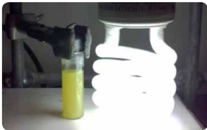
**Figure 3. Photoreactor Setup With a 26 W CFL Lamp**
