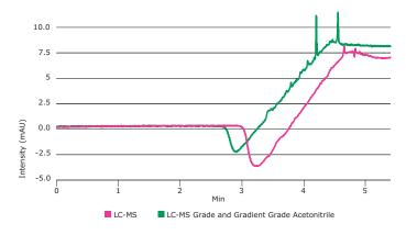
Blank runs of standard reversed-phase gradients of 30% to 80% acetonitrile in water generally result in low and stable baselines with HPLC columns packed with particles >3  $\mu$ m. However, this is not the case with UHPLC separations because of the typically higher flow rates and short columns. Performance tests conducted in ESI +/- ion mode using acetonitrile in water gradient show rising baseline for the blank gradient of standard HPLC grade solvents compared to LC-MS solvents.
