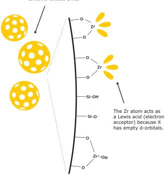
The phosphate moiety of phospholipids is a strong Lewis base (electron donor) that interacts with Zr atoms coated on the silica surface.
