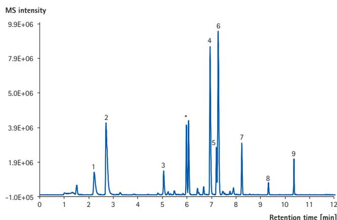
**Figure 3** LC-MS analysis of a tryptic digest of cytochrome c utilizing a monolithic silica capillary column.
