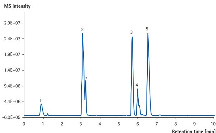
**Figure 4** LC-MS analysis of a mixture of five peptides on a monolithic silica capillary column.
