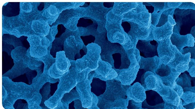
SEM image: Cross section of a silica monolith. Total porosity > 80%.
