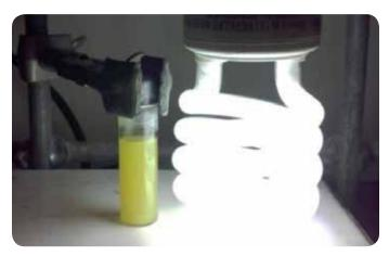
Figure 3. Photoreactor Setup With a 26 W CFL Lamp
